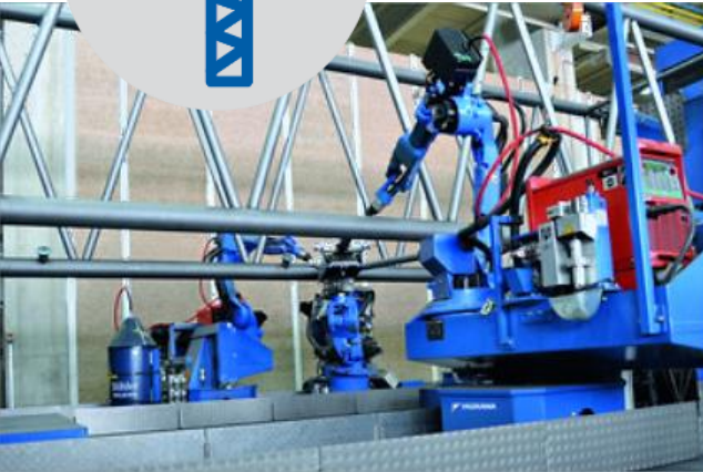
Fully automated welding of crane booms
